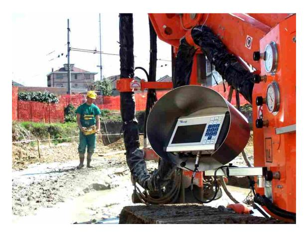
**JET-VISION** measurement system is a read-out and sensor device for the drilling and injection parameters used in **Jet-Grouting technology (mono-, bi- and triple-fluid).**
