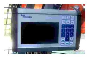
**MIX-VISION** measurement system is a new generation device used for the drilling and grouting parameters in the technology of soil mixing. It is based on Windows CE unit with a 7" color display. The system allows to measure and store the following parameters:
